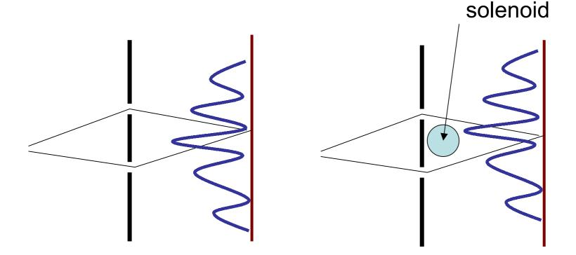
In a double slit interference experiment with electrons the interference fringes are shifted by the presence of a localized magnetic field by an amount proportional to the magnetic flux across the solenoid.
